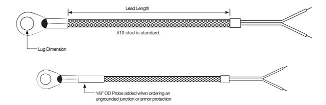
A ring lug thermocouple is used to measure surface temperature. A hole is drilled and tapped for a desired screw size. The screw is inserted through the lug and tightened down, securing the lug to the surface. A #10 stud is standard. Twenty gage wire is standard with most lug sizes.
