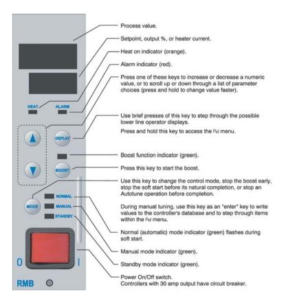
RMB controllers with the optional 30 amp output TRIAC are wider than the 15 amp units (to accommodate the heat sink), but the user interface is the same.
