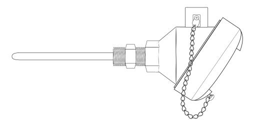
Protection head assembly are typically used in conjunction with a thermowell. The assembly can be mounted directly into the process or can be mounted into a thermowell, which is then mounted into the process.
