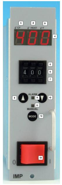
1 – soft start indicator – lit (orange) when soft start is active; flashes when controller is placed in standby by an external signal
