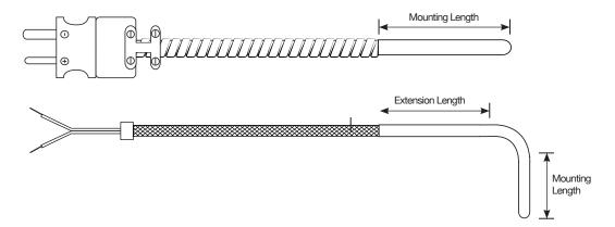
Fixed probe sensors can be used in drilled holes where mounting is not an issue. This type of construction can be submerged in liquids. Moisture proofing the lead exit is a popular option for immersion applications.
