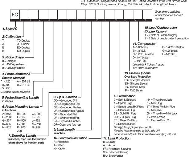
Fixed Compression, Type J, 90 Degree, 1/8" Diameter Probe, 3" Mounting Length, 1 1/4" Extension, Ungrounded Radius Tip, 96" Teflon Insulated Wire with Armor, Mini
