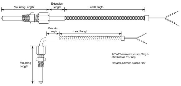
Another method of installing a thermocouple probe is by using it in conjuction with a compression fitting. After drilling and tapping the process hole, the compression fitting is threaded into the process and then tightened onto the probe, securing the probe in place. A brass 1/8" NPT is standard while others are available.
