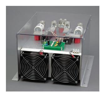
The Athena 19P (single phase) and 39P (three phase) are phase-angle fired power controllers that can be used for control of resistive heater loads. The high amperage series provides capacity from 125 amps up to 250 amps and the controllers are designed to extend heater life while eliminating thermal shock.
