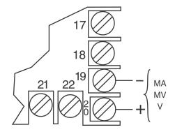
The Series C power supply accepts 100 to 250 Vac and 100 to 250 Vdc line power without any switch settings or polarity considerations. All connections should be made in accordance with the National Electrical Code and local regulations, using only NEC Class 1 wiring for all power terminals.
