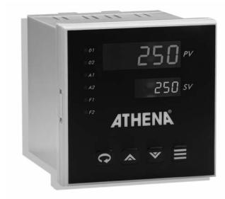
The Athena Legacy 25 is a 1/4 DIN panel mounted, auto-tuning controller that can be used for precise control of a single loop with two independent outputs. The controller accepts thermocouple, RTD, voltage, or current input. RS-232 or RS-485 communications are available, and two digital LED displays provide visual indication of various controller functions.
