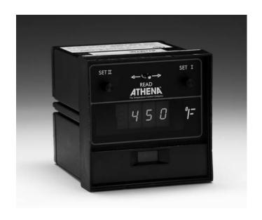
The Athena 4000 is a 1/4 DIN panel mounted, short metal case enclosed controller that can be used for accurate proportional temperature control of most processes. The controller accepts thermocouple or RTD input, and offers a choice of standard single outputs for energizing most common output devices. A single, digital filtered LED display provides visual indication of various controller functions.
