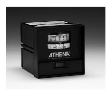
The Athena 2000 is a 1/4 DIN panel mounted, full featured, metal case enclosed controller that can be used for accurate proportional control of most processes. The Controller accepts thermocouple or RTD input and offers a choice of standard single outputs for energizing most common devices. A dual meter dial display provides visual indication of various controller functions.
